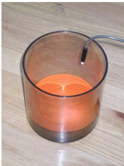
Figure 9: Apparatus for studying caustic curves with a light source inside the reflecting cylinder.
